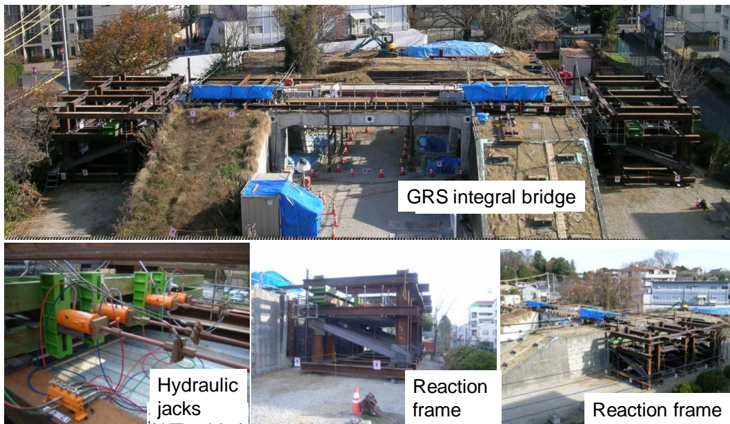
Figure 3. A general view of the model and arrangements for lateral loading tests
